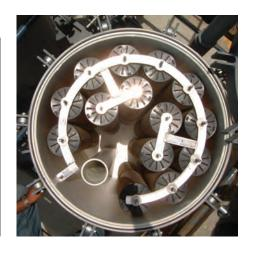
Parker Racor industrial HFP microfilters utilize proven and established cellulose media technology providing end users with a low cost, effective, and efficient dirt removal. HFP filters are typically employed in bulk fuel distribution systems to protect and prolong the life of water removal coalescers.
