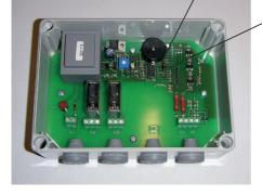
Jumper in pos 2 for both surface and high level alarm
