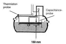
If a 1" cable gland is used for the mounting in the tank make sure that the cable is securely tightened. Make sure that the sensor is easy to lift out of the tank in order to protect the probe when emptying the tank.
