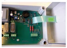
Make sure that foil connection is made correctly to the pin connector on the circuit board before the lid is closed.
