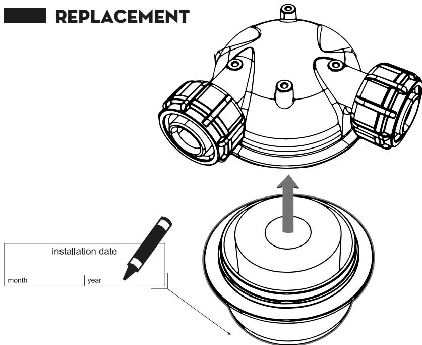
**EN.** Replace the filter with original spare parts every year or as necessary. Note the date of replacement.
