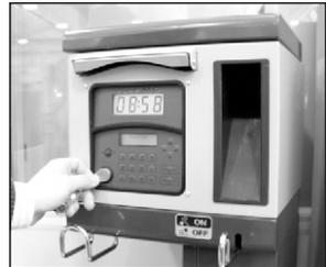
The stations to be used with USER KEYS with YELLOW key holder indicate the software release of the station in the second line of the alphanumeric display (ex. ver. 3.0).
