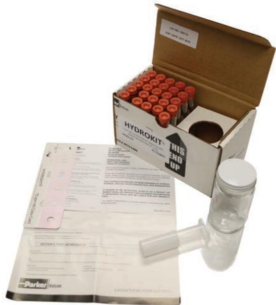
The HYDROKIT provides better water determination than ASTM D2709 or D4176. The HYDROKIT is designed for “fail-safe” operation, with false negative readings unlikely. Almost any error in performing the test will indicate the presence of wet fuel. If the sample indicates the presence of excessive water, it is always a good practice to repeat the test on a second sample.
