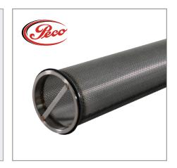
The XtreamPure, Series XP-SS, is a large 6" diameter strainer designed to flow liquid from inside-to-outside. This design has several advantages. It keeps contaminants trapped within the strainer, so the vessel remains clean. The strainer includes a handled
