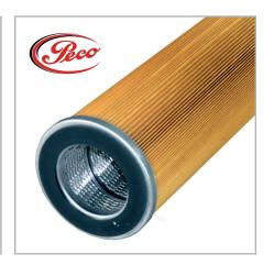
Series S separator cartridges are used in conjunction with Series C and IPC coalescer cartridges in vertical and horizontal PECO Series 110 vessels. They can also be used as a retrofit to other competitor equivalents. The cellulose media is hydrophobic and the cartridge acts as a final check to repel coalesced water droplets and prevent them from going downstream.
