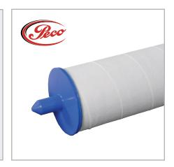
The PEACH Gemini, Series PGC, cartridge is specifically designed for use with the PEACH Gemini PuraSep vessel in natural gas filter-coalescing applications. Its unique patented design provides dual flow path filtration with all the added benefits of PEACH technology. Gas flows outside-to-inside through the 1st Stage of the cartridge where
