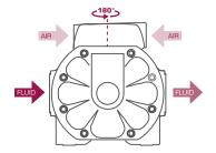
Orientable air inlet, increased installation flexibility.
