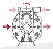
Orientable air inlet, increased installation flexibility.
