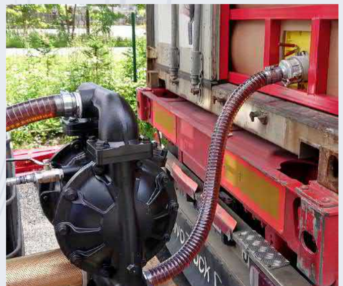
High fluid viscosity reduces pump delivery.
