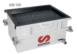
**439 100 Pit rolling drainer**, **95 Litres** Rolling drainer for being installed between pit rails with minimum / maximum width of 1.040 / 1.450 mm. 95 litres (25 US gallons) capacity. Unit includes antisplash grid, four vertical and four horizontal rollers for easy rolling and an 1-1/4" outlet with ball valve. The unit allows the connection of a hydraulic connector for discharging with a discharge pump kit.
