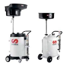
**Gravity collection with pump discharge.** Discharge is done through a 1:1 pressure ratio pneumatic piston pump attached to the back of the unit reservoir and 1,5 m hose with a hydraulic type coupler.
