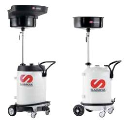
**Gravity collection with pressure discharge.** Discharge is done through a 1,5 m hose pressurizing the unit at 0,5 bar (3.5 psi). Includes a safety valve to avoid over pressurization.
