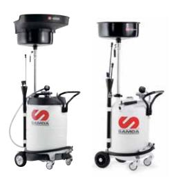
**Combined waste oil suction and gravity collection units.** They can be used remotely once vacuum is created inside the steel reservoir. Discharge is done through a 1,5 m discharge hose pressurizing the unit. Includes safety valve to avoid over pressurization.
