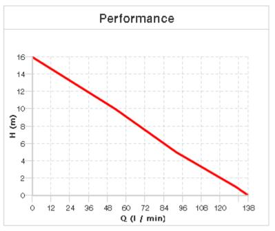
Characteristics referring to operation with water at  $20^\circ\text{C}$
