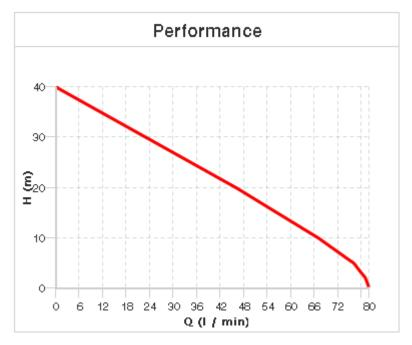
Characteristics referring to operation with water at 20  $^{\circ}\mathrm{C}$
