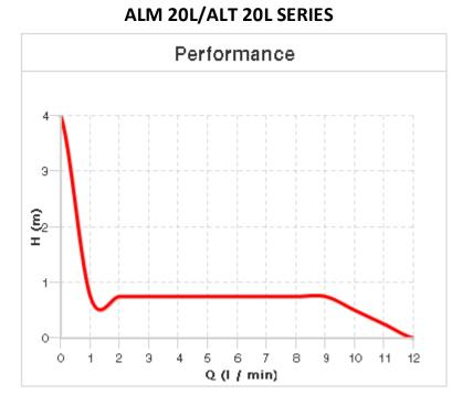
Characteristics referring to operation with water at 20°C
