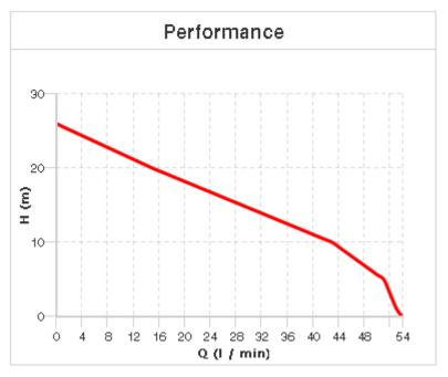
Characteristics referring to operation with water at 20  $^{\circ}\mathrm{C}$
