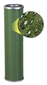
Coalesced water drops from the first stage are shown (above) intruding upon the surface of the PCS Separator Cartridge. The droplets are repelled by the PTFE coated screen, enabling the droplets from passing through. The screen magnification shows how the droplets form on the surface of the PTFE coating.
