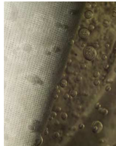
Coalesced water drops releasing from the knitted sock at the outside surface of the cartridge.
