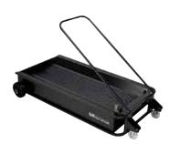
Low level mobile drainers for gravity collection of waste oil and used automotive fluids such as antifreeze solutions. Recommended to use when a hoist or a service pit is not available. Gravity discharge through a drain valve or using an evacuation pump kit (PN 559 100) through a dry break hydraulic connector (PN 950 352) (not included).
