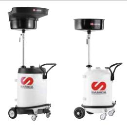
**Gravity collection with pressure discharge.** Discharge is done through a 1,5 m hose pressurizing the unit at 0,5 bar (3.5 psi). Includes a safety valve to avoid over pressurization.
