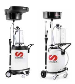
Combined waste oil suction and gravity collection units, with transparent chamber. Units with a 10 litres transparent chamber that can be used as a vacuum reservoir and allows an immediate inspection of the extracted waste oil. They can be used remotely once vacuum is created inside the steel reservoir. Discharge through a 1,5 m discharge hose pressurizing the unit. Includes safety valve to avoid over pressurization.
