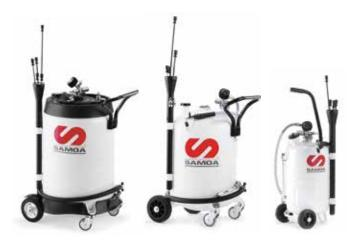
**Waste oil suction collection units.** They can be used remotely once vacuum is created inside their steel reservoir. Discharge through a 1,5 m discharge hose pressurizing the unit (except model 371 600). Includes safety valve to avoid over pressurization.
