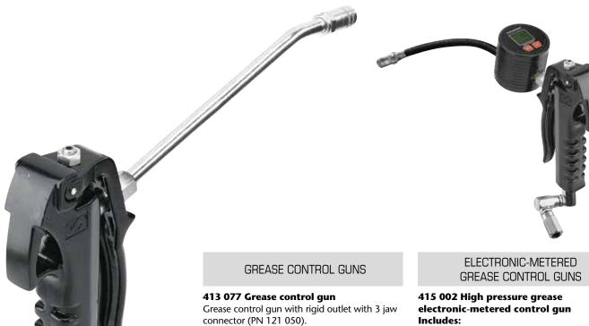
High pressure grease control guns with ergonomic body and trigger designed to reduce operator hand fatigue. Manufactured in aluminium with steel insert for high pressure. Maximum working pressure: 500 bar (7,150 psi). Inlet thread: 1/4" BSP (F).
