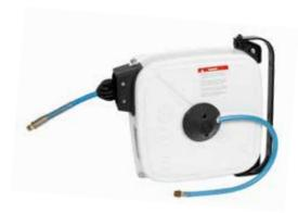
Compact enclosed reels for compressed air, manufactured in steel. All reels include pivoting wall bracket for an easy and convenient installation. Reels are supplied with PVC hose and they have a maximum working pressure of 15 bar (285 psi).
