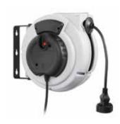
**612 400** - **230 V, 50 Hz cable reel with 230 V AC to 24 V DC transformer with LED lamp.** 15 m H05RN-F 2x1 mm<sup>2</sup> cable hose reel. Includes a 230 V AC to 24 V DC transformer and a 900 LUMEN LED light.
