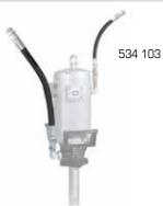
**534 103** Includes 1 m x 3/8" air hose (PN 247 710) with 3/8" - 1/2" BSP (MM) connection threads, quick air coupler 251 438, air nipple 255 338, 1,5 m x 3/8" high pressure grease hose (412 392) with 3/8"-1/2" BSP (MM) connection threads. For use with all PM45 and PM60 grease pumps except with pump PM60 12:1 ratio grease pump.
