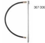
Suction assemblies for wall mounted stub pumps. Assemblies include Ø 42 suction tube with foot valve, height adjustable 2" bung adaptor and 2 m x 1" rubber connection hose.
