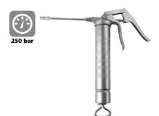
Pistol grip grease pump for hard to reach lubrication points. Three way loading: 400 g (14 oz) cartridges, bulk grease suction or filler pump. Heavy duty cast iron head with precision fit piston. Maximum working pressure: above 250 bar (3,650 psi).
