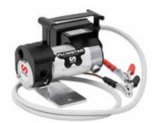
External gear pumps with 12 and 24 V DC motors wit IP55 protection, on/off switch, fuse and 2 m cable with crocodile clamps. Pump can work in interment duty cycles of 30 minutes and has built in by-pass valve.
