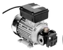
Internal gear electric pumps for lubricants. 230 V - 50 Hz (single phase) or 400 V - 50 Hz (three phase) motor depending on model, IP-55 protection and on/off switch. Cast iron pump body, sintered steel gears and by-pass valve. Motor with mounting feet, the pump can be mounted horizontally on a flat surface or vertically to a wall.
