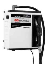
50 or 70 l/min Polaris Series pump in a cabinet for wall or tank mounting. The unit includes a 230 V - 50 Hz diesel pump with 1,8 m cable with plug, cabinet with nozzle holder with automatic on/ off switch, 4 m delivery hose, automatic nozzle and a three digit meter, flange mounted to the pump and with a 90° swivelling elbow outlet.
