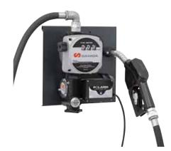
50 or 70 l/min Polaris Series pump on a bracket for wall or tank mounting. The kit includes a 230 V - 50 Hz diesel pump with on/off switch and 1,8 m cable with plug, wall mounting bracket, 4 m delivery hose, nozzle and a three digit meter (PN 680 300) flange mounted to the pump and with a  $90^{\circ}$  swivelling elbow outlet. Fluid inlet connection 1" BSP (F).
