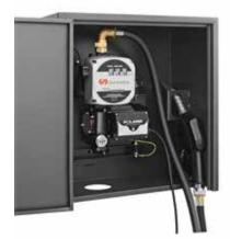
50 or 70 l/min Polaris Series pump in a cabinet with safety lock for wall or tank mounting. The unit includes a 230 V - 50 Hz diesel pump with 1,8 m cable with plug cabinet with nozzle holder with automatic on/ off switch, 4 m delivery hose, automatic nozzle and a three digit meter, flange mounted to the pump and with a  $90^{\circ}$  swivelling elbow outlet.
