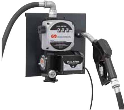
50 or 70 l/min Polaris Series pump on a bracket for wall or tank mounting. The kit includes a 230 V - 50 Hz diesel pump with on/off switch and 1,8 m cable with plug, wall mounting bracket, 4 m delivery hose, nozzle and a three digit meter (PN 680 300) flange mounted to the pump and with a 90° swivelling elbow outlet. Fluid inlet connection 1" BSP (F).
