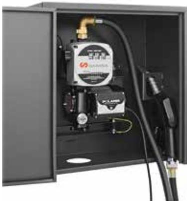
50 or 70 l/min Polaris Series pump in a cabinet with safety lock for wall or tank mounting. The unit includes a 230 V - 50 Hz diesel pump with 1,8 m cable with plug cabinet with nozzle holder with automatic on/ off switch, 4 m delivery hose, automatic nozzle and a three digit meter, flange mounted to the pump and with a 90° swivelling elbow outlet.
