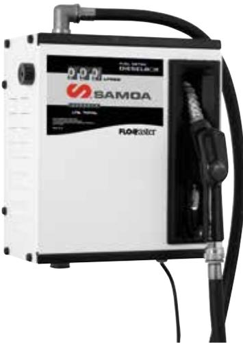
50 or 70 l/min Polaris Series pump in a cabinet for wall or tank mounting. The unit includes a 230 V - 50 Hz diesel pump with 1,8 m cable with plug, cabinet with nozzle holder with automatic on/ off switch, 4 m delivery hose, automatic nozzle and a three digit meter, flange mounted to the pump and with a 90° swivelling elbow outlet.
