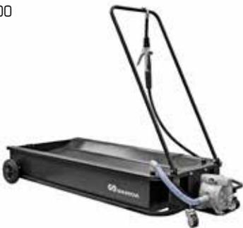
Low level mobile drainers for gravity collection of waste oil and used antifreeze solutions. Recommended to use when a hoist or a service pit is not available. Gravity discharge using an evacuation pump kit (PN 559 100) through a dry break hydraulic connector (PN 950 352, not included).
