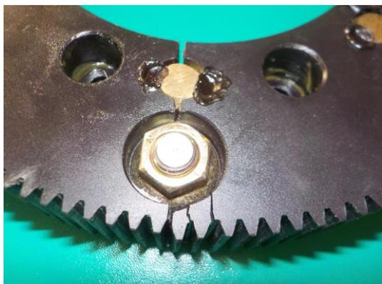
*The divided replacement gear is too tight during installation to the area of the tooth pitch segments → the distance of the tooth does not fit in the two separation points.
