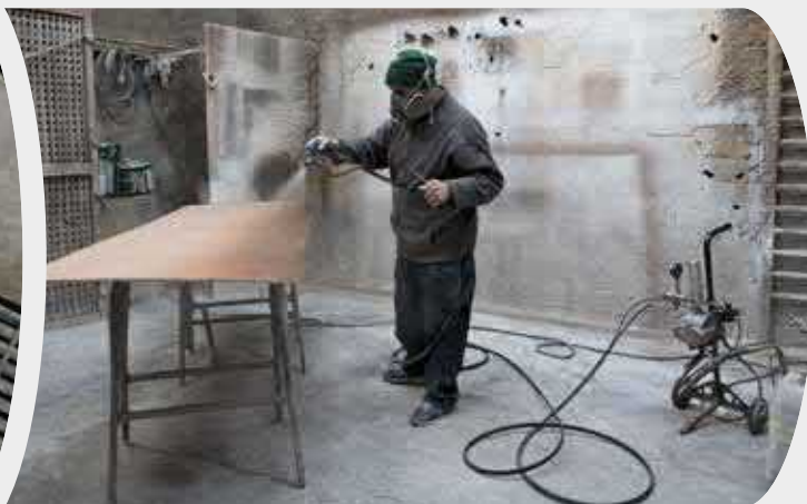
Wood varnish spraying.
